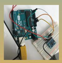
Evan suggested that I test out the gyroscope to make sure it's functioning properly. This step is one way of preventing time wastage. It was also an encouraging sight to see that the project is on its way. I used a Serial.println () to monitor the numbers and angles.
